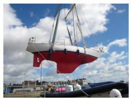
of the keel which had some 20 laminations of 2oz GRP matting applied as filler and strengthening with a couple of layers of Gel Coat to give a smooth, watertight finish. In the immortal words of Dave Saunders of 'Wavetrade' who undertook the repair, 'The new reinforced GRP keel shoe should outlast the yacht...'
